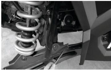
3. Drill out original hole in trailing arm and brake line mount to 1/4 ". Use pliers to securely hold the brake line mount while drilling.
