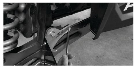
10. Tighten all hardware. Instruction apply to both the driver and passenger side of vehicle.
