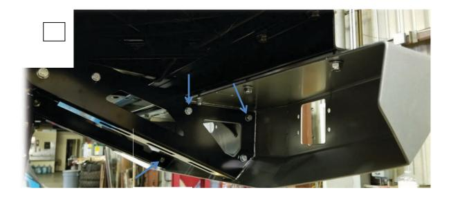
7. Raise the bumper up against the previously installed bed adapter bracket and install the 8) M8-1.25x20 button socket head bolts in through the top of the bracket as shown below, with M8 flat washers and M8-1.25 locknuts underneath.
