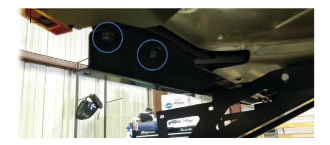
6. Slide winch bumper into place. Align interior mounting brackets of the bumper inside the previously installed mounting arms. Thread the 8) M8-1.25x16 hex head bolts with M8 flat washers through the slotted holes of each of the mounting arms and into the threaded holes of the bumper as shown in Image F. Do not tighten any hardware at this time.
