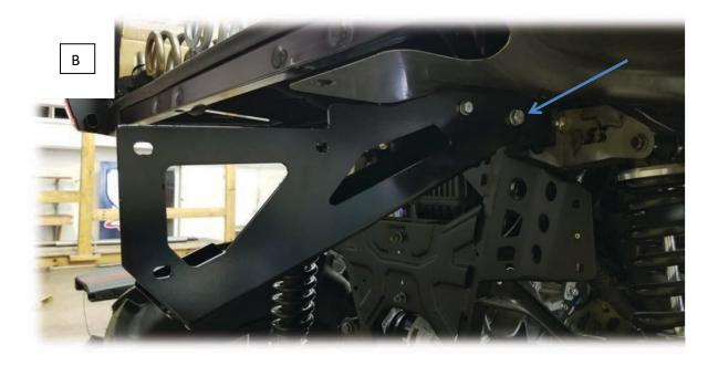
Install an M10 flat washer and M10-1.5 locknut onto new bed pivot bolt. Install the 2) M81.25x20 hex head bolts, M8 flat washers, and M8-1.25 locknuts through each rearmost hole of
