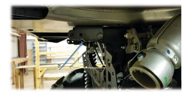
Slide the winch bumper passenger side mounting arm over the outside of the OEM bed
