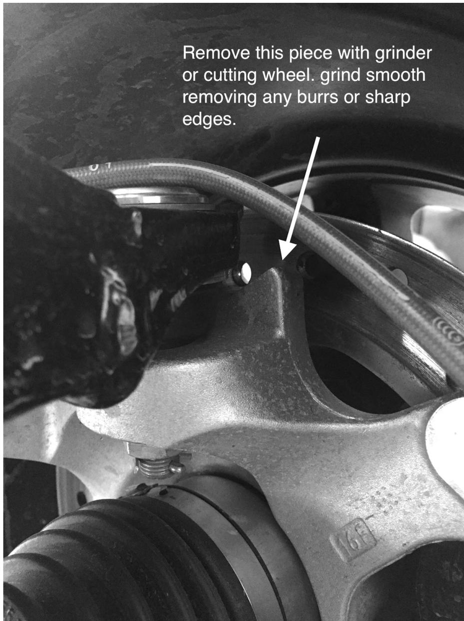
Remove this piece with grinder or cutting wheel. grind smooth removing any burrs or sharp edges.
